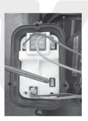
Step 6 – Connect the communication cable the main board of the Electrochlor into the Waterco ECO pumps socket.
