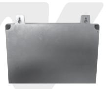
2. To access the Electrochlor for connection of cabling and sensors, there are screw wells in each corner of the front panel. To open the panel, insert a flat blade screw driver and half turn anti-clock wise to release the spring loaded locking pin. Ensure the pins are fully released prior to opening the hinged front panel.
